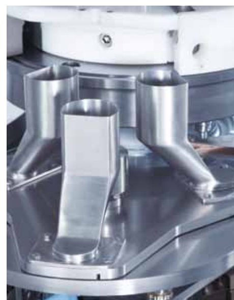
Automatically rotating filling wheel
