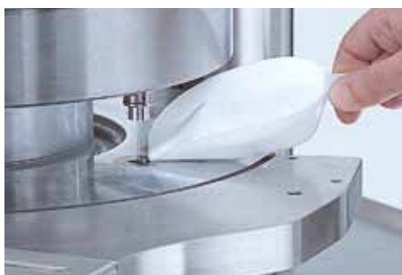
Manual filling for single punch compression
