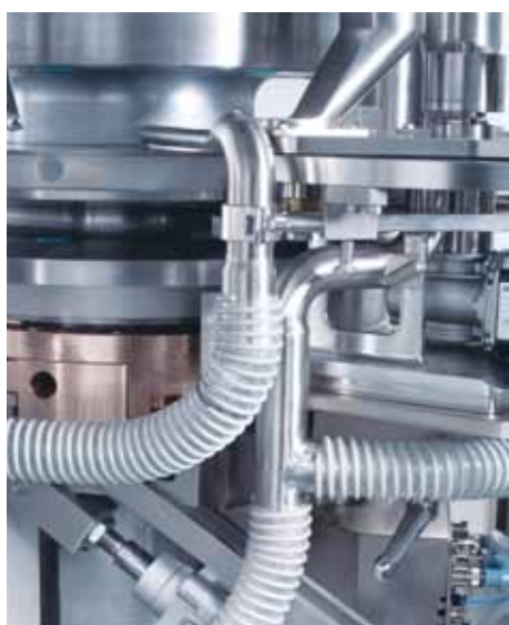
Dust extraction for multi-layer tablets
