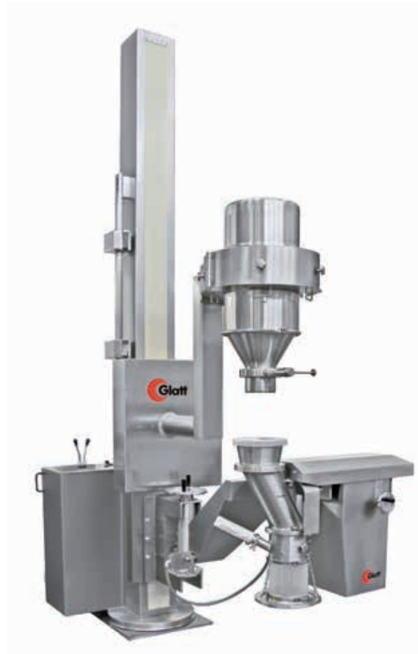
EL 600 lifting device for discharging drums through a GS 180 rotor sieve
