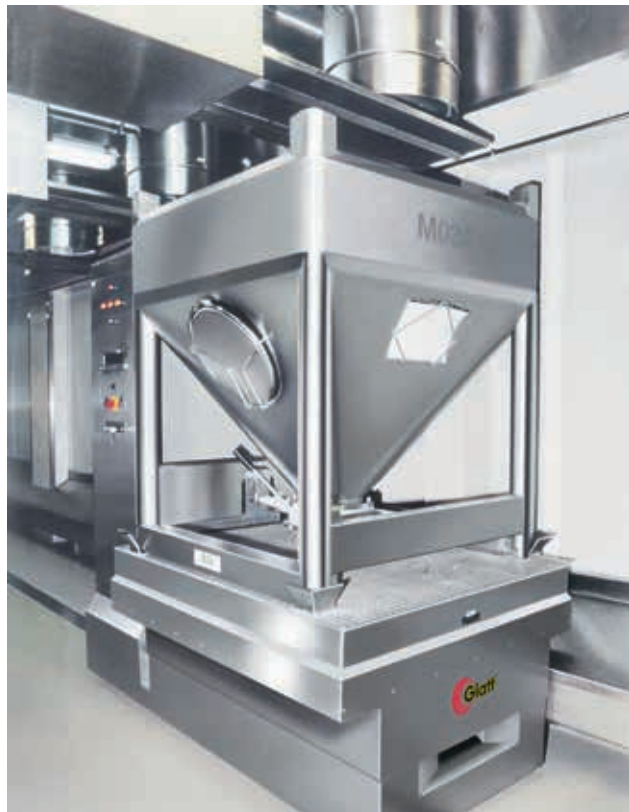
Automatic weighing and charging of ICBs
