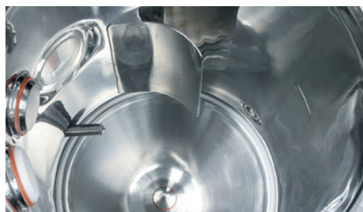
Pelletizing in the CPS insert
