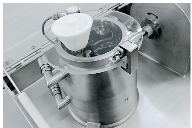
TMG 1 l working vessel with funnel and temperature sensor
