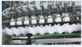
Bottle Mouth Holders: The dedicated bottle holders are required when bottle mouth opening is too small to be centered and aligned with fill nozzles.
