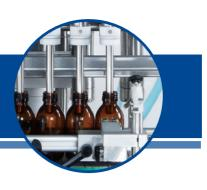
CVC 3036-8 with in-line configuration are really versatile fillers that easily - and inexpensively - accommodates to different bottle sizes.
