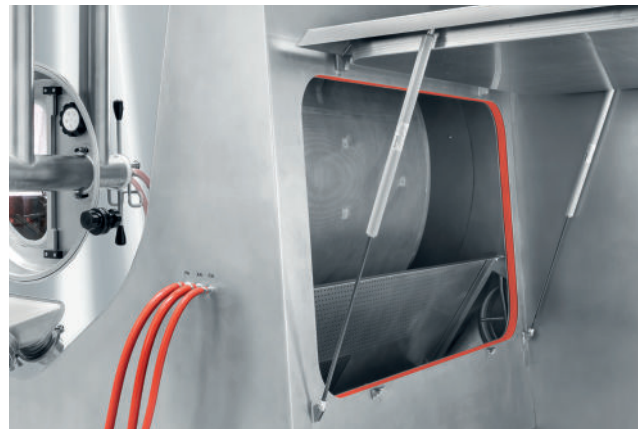
Inlet air diffuser with inflatable seal
