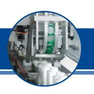
The CVC 1206 Capper is a very flexible machine designed to apply and tighten screw-on caps onto containers at rates of up to 140 bottles per minute. The CVC 1206 is Siemens PLC controlled. The system is designed with three pairs of capping spindles. Options include tower lamp, hopper level control, cap inspection (level cap, foil seal, and no cap), reject, and reject verification.
