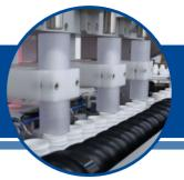
The CVC 1117H of Cotton Inserter is designed to insert polyester, rayon, or cotton coil into containers at speeds up to up to 200-210 bottles per minute. The CVC 1117H is Siemens PLC controlled and Servo Motor driven. Options include tower lamp, missing cotton in bottle detection, reject, and reject verification. The cotton piece length can be set from 60mm to 150mm.
