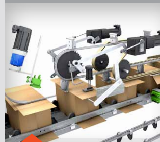
case squaring and compression for sealing case
