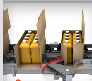
flap tucker timing and motion
