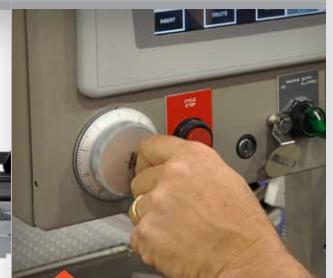
handwheel control for optimizing set points
