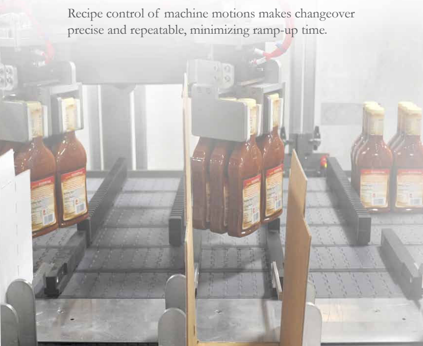
case squaring and compression for sealing case
