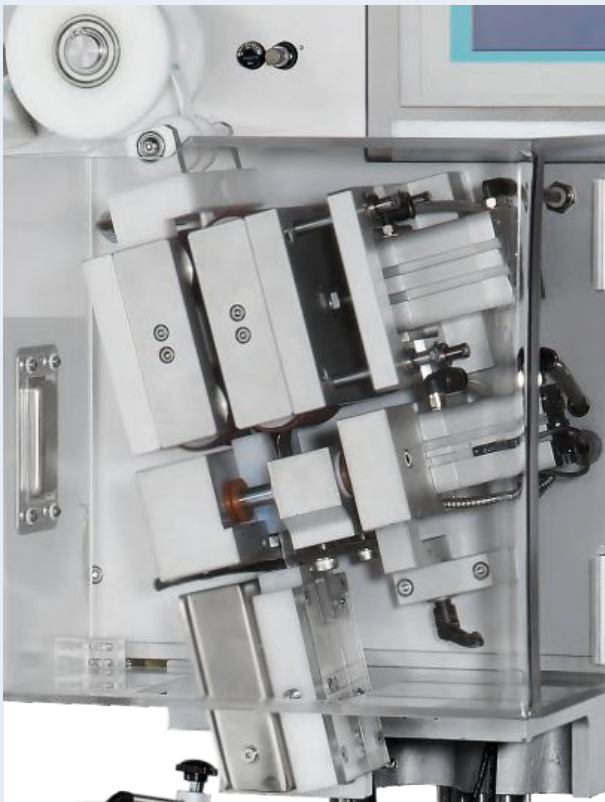
• Pouch Desiccant Cutting and Dispensing Mechanism
