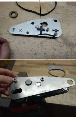
8. Inspect both brass sprockets and all six (6) bearings for any damage, looseness or things stuck on them. Replace when needed;
