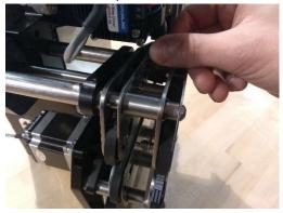
3. Remove carefully the connector from the top driving stepper motor;
