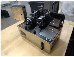
3. With a pair of nose pliers, dislodge the two (2) springs from the bottom belt holder assembly;
