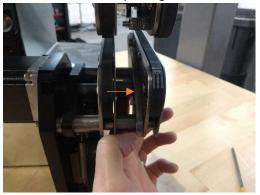
21. Now, check the tension of the new belts. If needed, tension it by the bottom head screws behind each holder. An Allen key 1/8 90 degrees is required;
