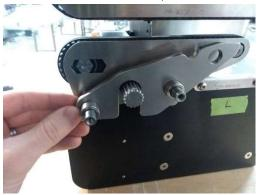
17. Continue with the next assembly. Like the other one, inspect the sprocket and the bearings. Replace if needed;
