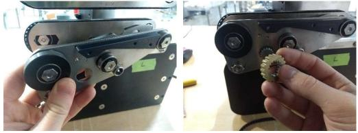
18. Replace the front belt. Tensioning will be done later. <u>Careful</u>, there is two size of belt;
