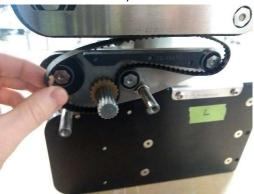
13. As the first holder, inspect the sprocket and the three (3) bearings for any damage, looseness, no plastic from bags or product are stuck on them. Replace if needed;
