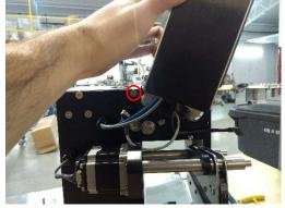
6. Take off the top frame. If it is too tight to remove, loosen a quarter turn or these flat head screws (remember to retighten them);
