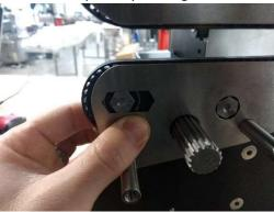
16. Insert the spacers and the bevel part, but leave the set screws for later;
