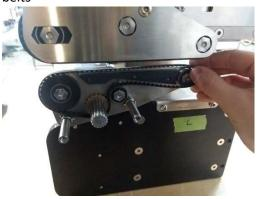
15. Put back the plate by making sure the bearing nut is well engaged into it
