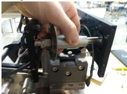
8. Remove the jewelry saw with a 3/4 wrench. Make sure the teeth will be oriented down as shown;
