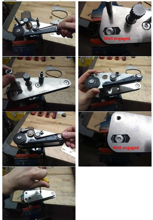
10. Now, check the tension of the new belts. If needed, tension it by the bottom head screws behind each holder. An Allen key 1/8 90 degrees is required;
