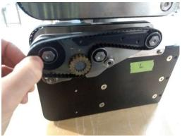
7. Remove the sprocket from the spline shaft.
