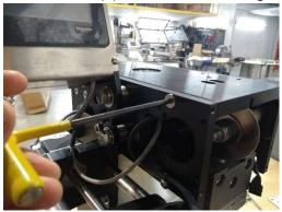
5. For the last screw, the two (2) hexagonal screws of the screen bracket need to be loosen with a 9/16 wrench;
