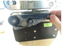
19. Put back the front plate, make sure the bearing nut is well engaged into the plate and tight it with the screws;
