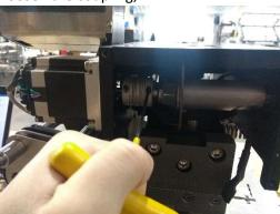
5. Unplug gently the feeder motor connector and unscrew the four (4) screws of the motor **Careful:** These motors are fragile to impact, avoid dropping them.
